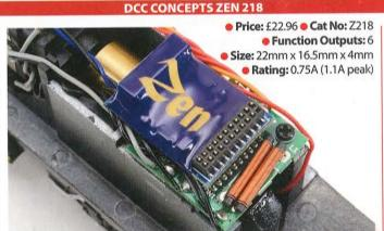
lighting effects, Back EMF, short and long addressing, advanced consisting and it comes with a separate 'stay-alive' capacitor, which can be soldered to the decoder via the attached blue and black wires. Lighting effects include a fluorescent flicker, useful for modern style locomotives and units, and firebox flicker too. Acceleration, deceleration and
